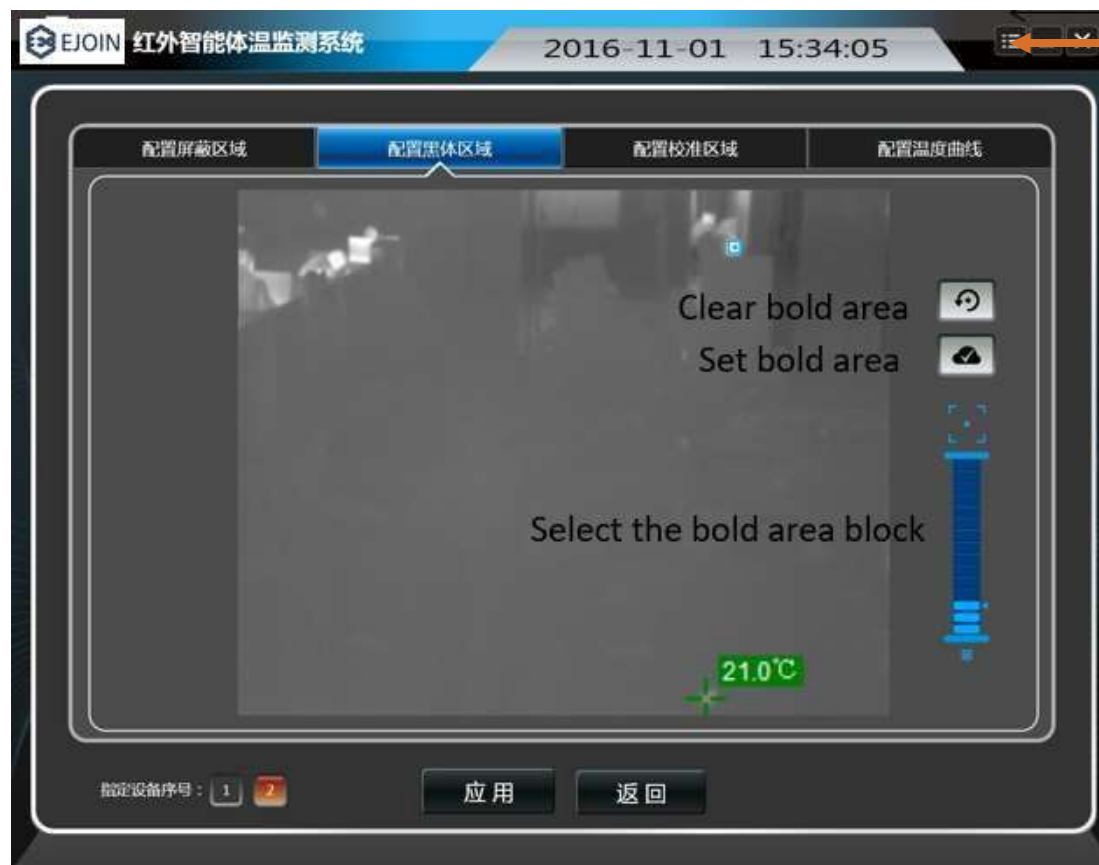
Temperature Measurement Parameter Registration-Blackbody Region
